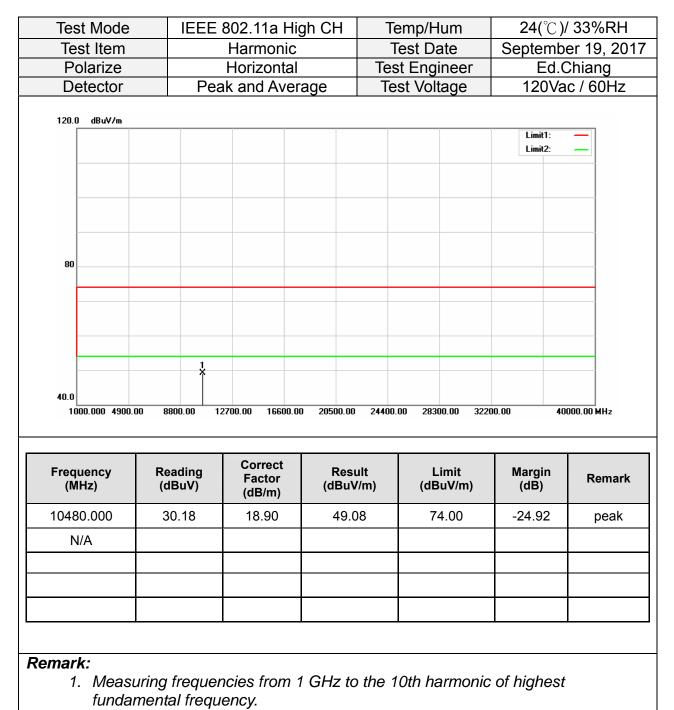
2. For above 1GHz, the EUT peak value was under average limit, therefore the Average value compliance with the average limit
