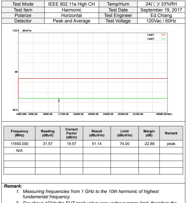
2. For above 1GHz, the EUT peak value was under average limit, therefore the Average value compliance with the average limit
