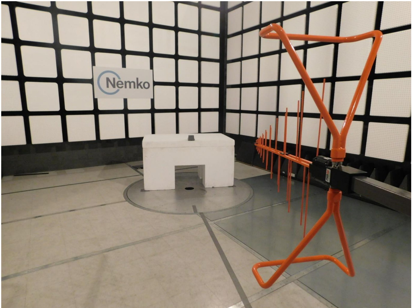
Radiated 30 MHz – 1 GHz ALF-000044 (Flowie)
