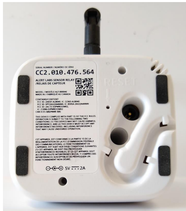
Figure 2: Sensor Relay Bottom View, Host Label Location (shown on ALF-000046)
