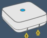
**2** Test it out. Check for a blue light as you hold a kitchen knife across both metal contacts at the same time to simulate a flood.
