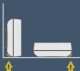
**3** Remove the installation sticker. Place your Floodie on the floor or stick it to the wall. Keep the metal contacts against the floor.
