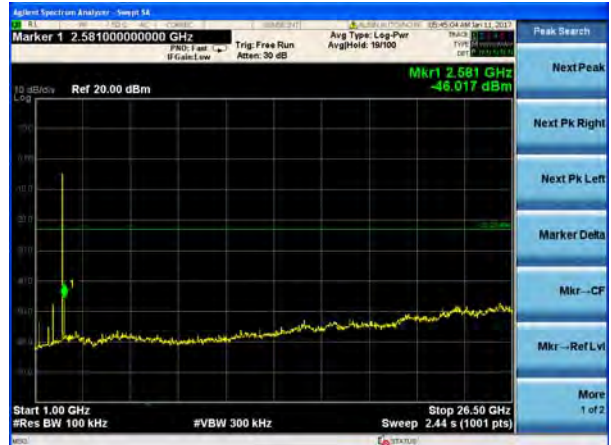
GFSK on channel 39
