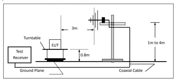
(c) For radiated emissions above 1000MHz
