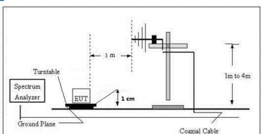
30-1000MHz Test Setup
