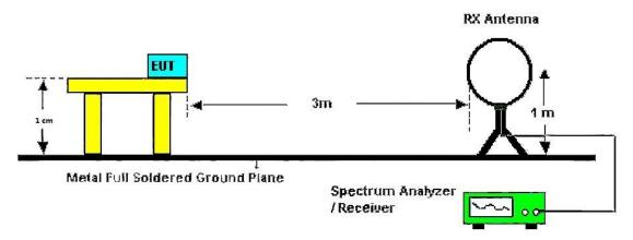
Below 30MHz Test Setup
