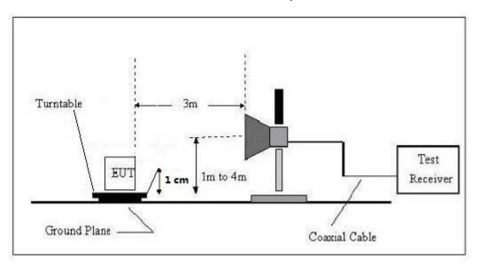
Above 1GHz Test Setup
