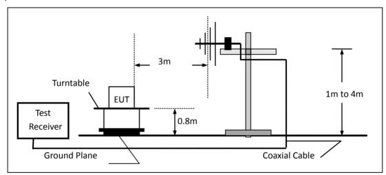
(c) For radiated emissions above 1000MHz
