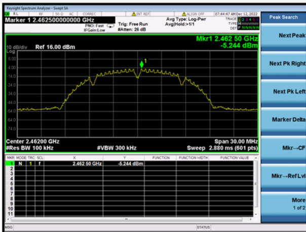
802.11b HIGH CHANNEL, CARRIER LEVEL
