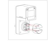
2. Confirm the place of installation and direction of the SwitchBot Lock. Confirm the following based on the position of vour lock and handle:
