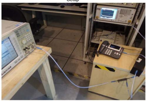
Frequency Stability Under Temperature & Voltage Variations Setup
