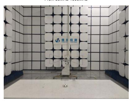
Test frequency from 1GHz-18GHz
