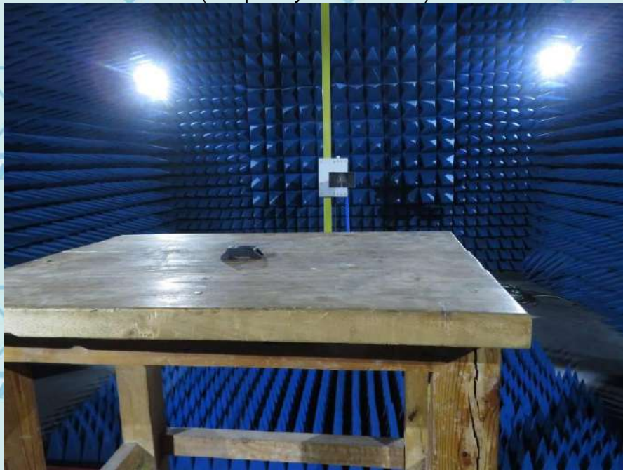
RADIATED EMISSION TEST (Frequency above 1GHz)
