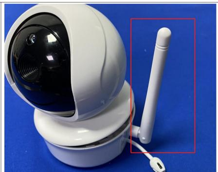
The antenna is External antenna. The best case gain of the antenna is 3dBi.
