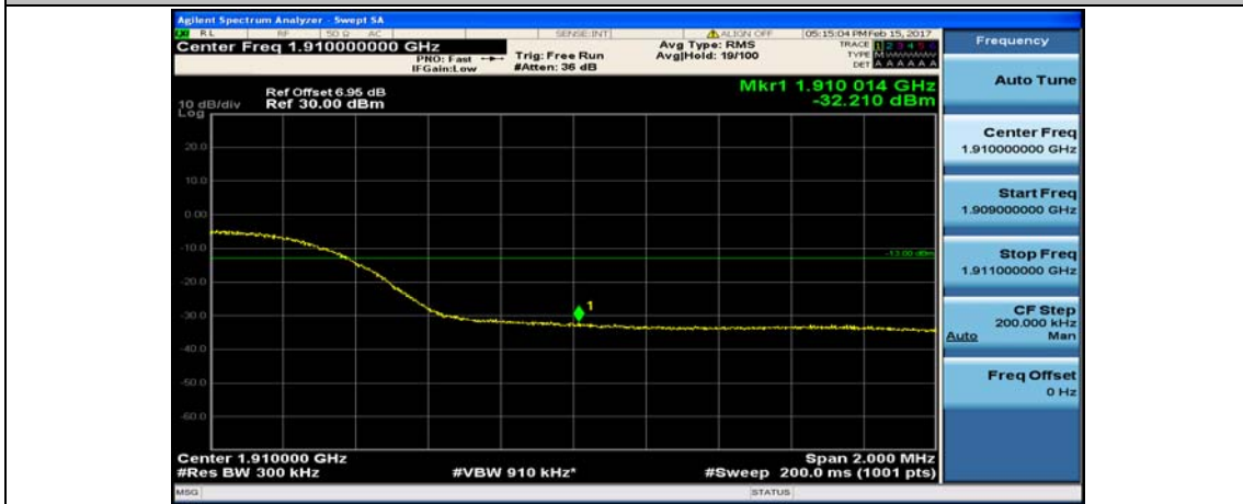
(Channel Bandwidth:15 MHz)_HCH_16QAM_75RB#0
