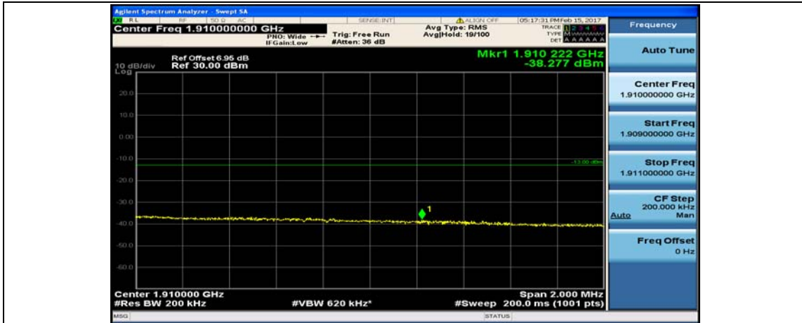
(Channel Bandwidth:20 MHz)_HCH_16QAM_50RB#50
