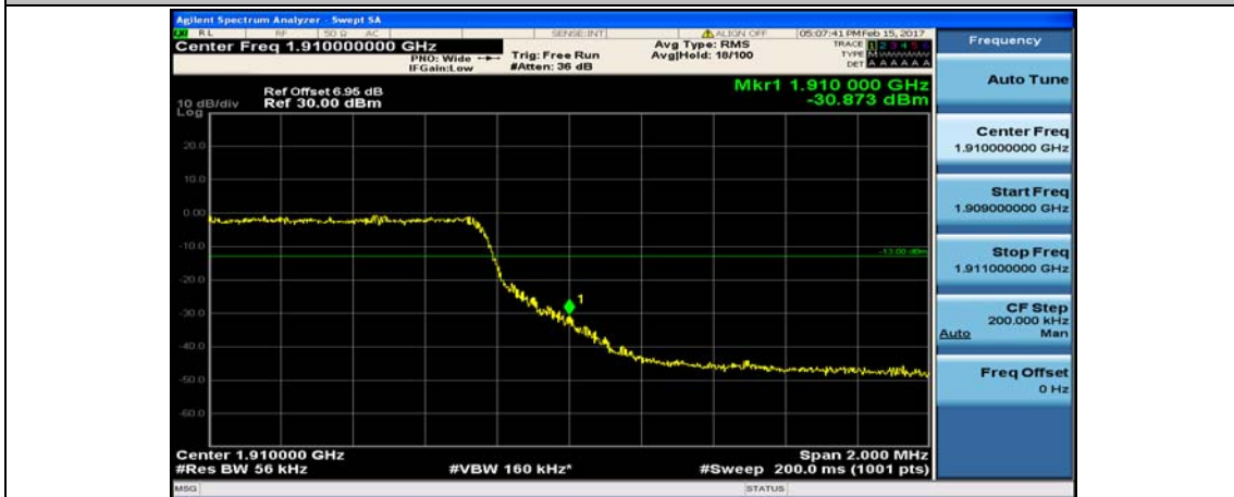
(Channel Bandwidth: 5 MHz)_HCH_QPSK_25RB#0
