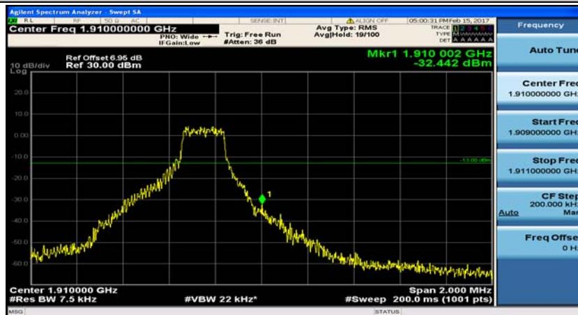
(Channel Bandwidth: 1.4 MHz)_HCH_16QAM_3RB#0
