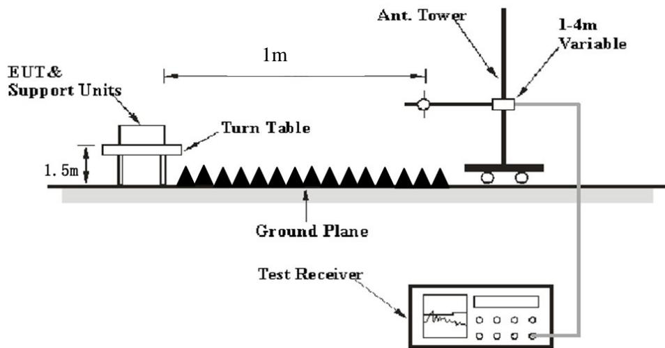
The radiated emission tests were performed in the 3 meters chamber, using the setup accordance with the ANSI C63.10-2013. The specification used was the FCC 15.209, and FCC 15.517 limits.
