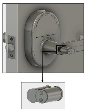
Once the removable core is aligned, insert the key and turn clockwise 15 degrees to retract the catch, then insert the core into the lever. Turn the key back counterclockwise 15 degrees to engage the core and remove the key.
