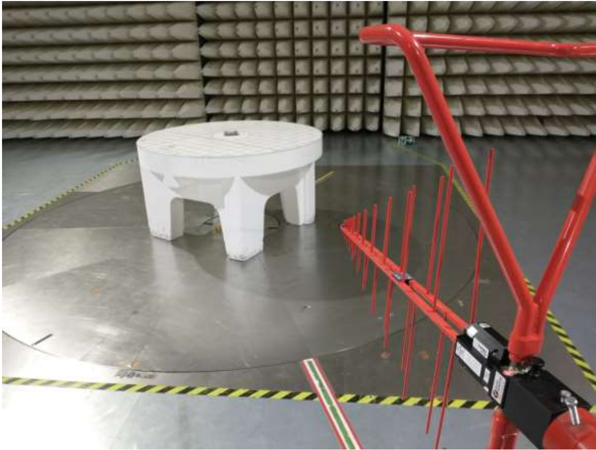
Figure 27. 30-1000MHz Radiated Test Setup
