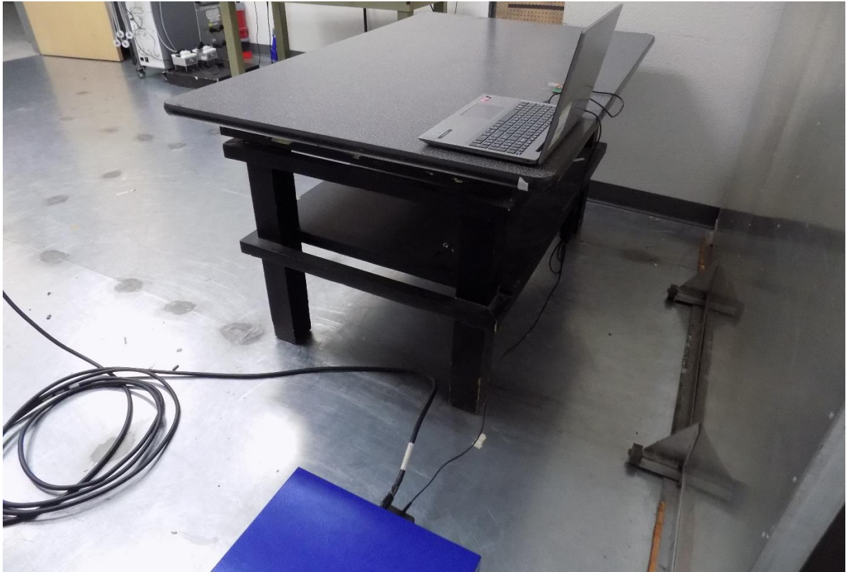
Figure 2: Test Setup for Conducted Emissions – Rear View
