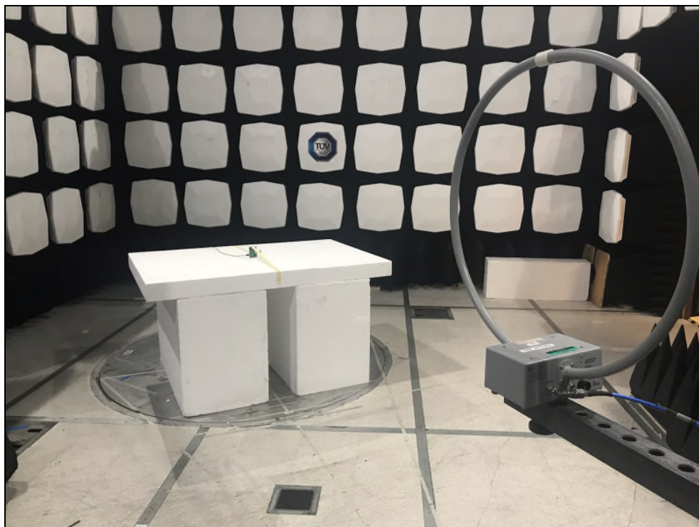
Figure 6: Equipment Under Test – Radiated Emissions <30MHz
