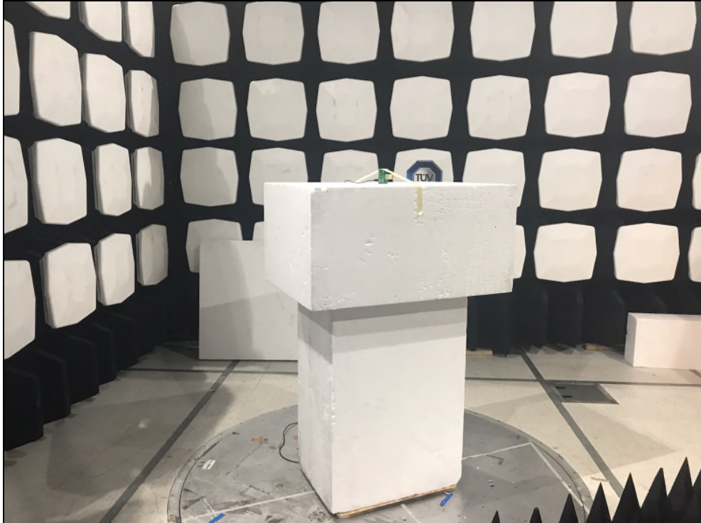
Figure 10: Equipment Under Test – Radiated Emissions >1GHz
