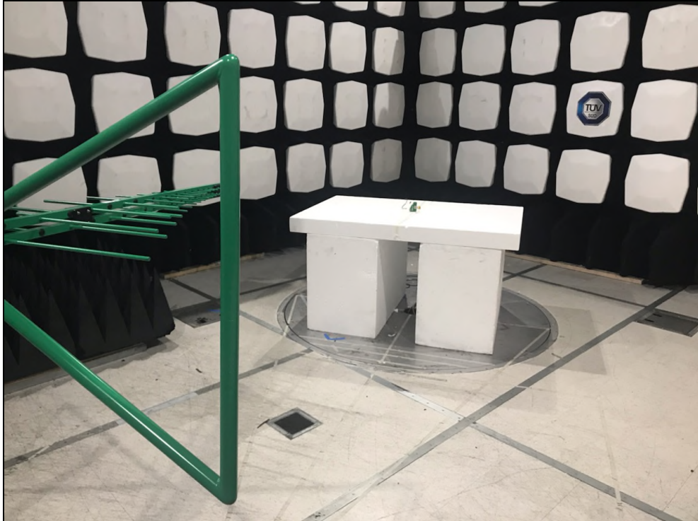
Figure 8: Equipment Under Test – Radiated Emissions <1GHz
