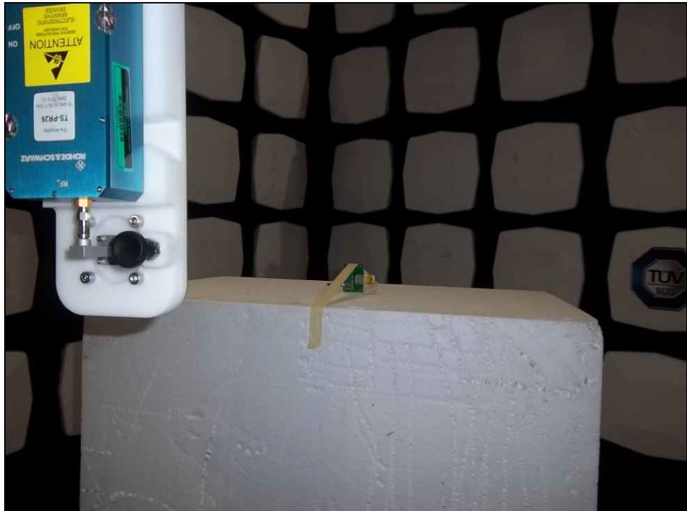
Figure 12: Equipment Under Test – Radiated Emissions >18GHz
