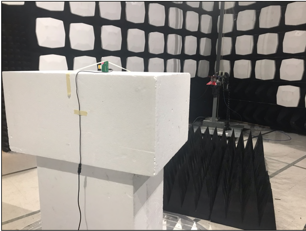
Figure 11: Equipment Under Test – Radiated Emissions >1GHz
