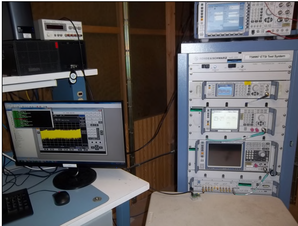
Figure 1: Equipment Under Test – Antenna Port Conducted Measurements
