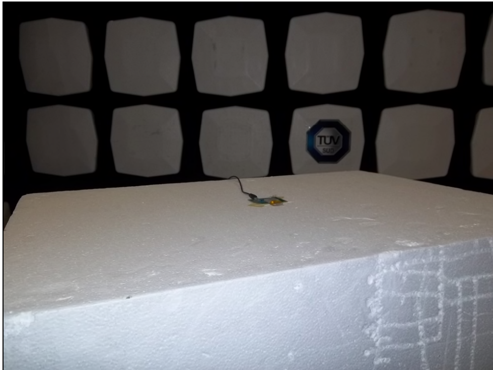
Figure 5: Equipment Under Test – Radiated Emissions Z-orientation
