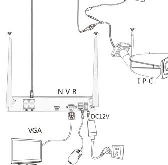
After power on, the system starts and automatically connects the wireless IPC
