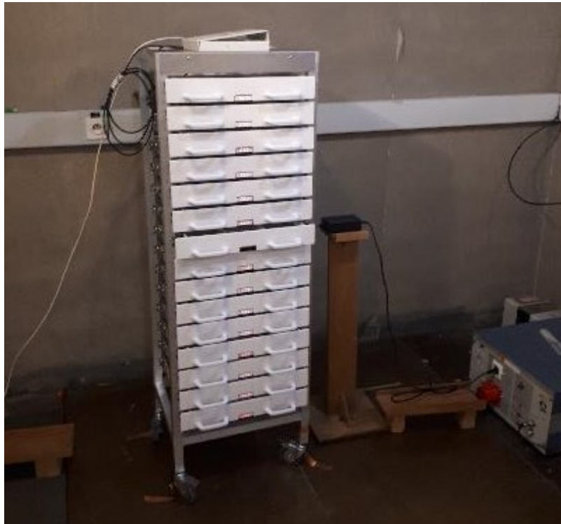
Photograph for AC Power Line Conducted Emissions (Front view)
