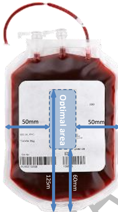
Figure 9 – Position of the tag on the bag for optimal RFID reading
