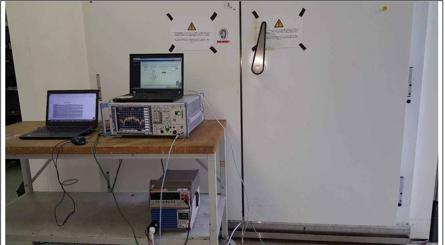
Photograph for Frequency Tolerance in extreme test condition
