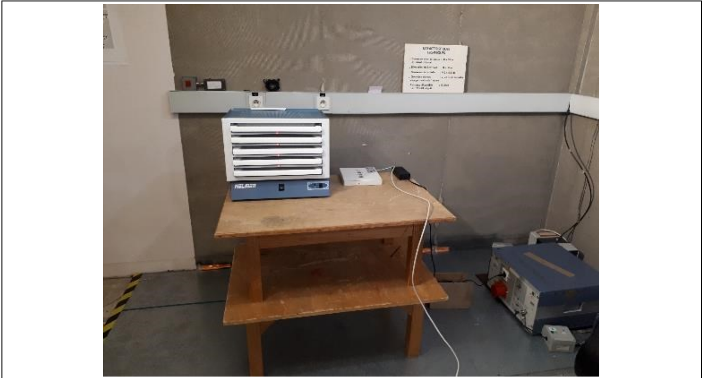
Photograph for AC Power Line Conducted Emissions (Front view)
