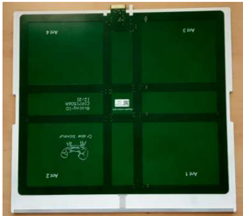
Satellite bottom without lexan (plastic adhesive)
