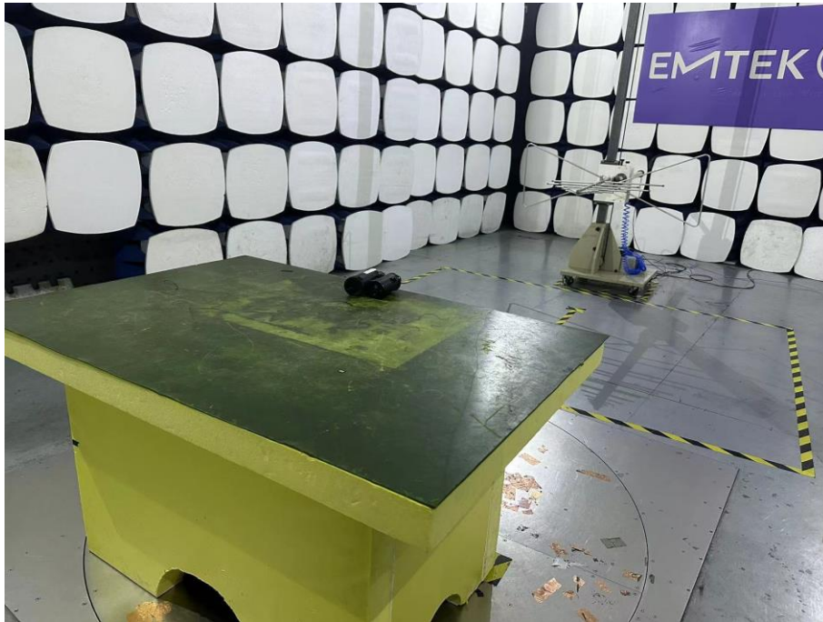
Spurious Emission Test Setup (Below 1GHz)
