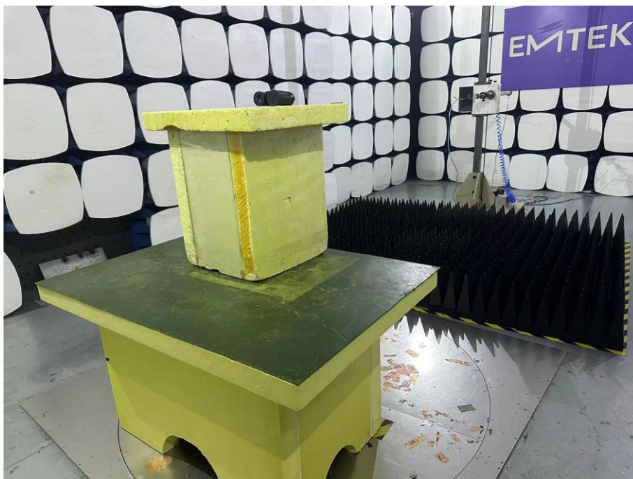
Spurious Emission Test Setup (Above 1GHz)
