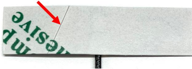
1. Find cut line on flex back side
