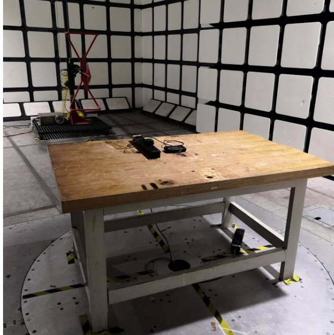
Radiated Emissions View (Below 1 GHz)
