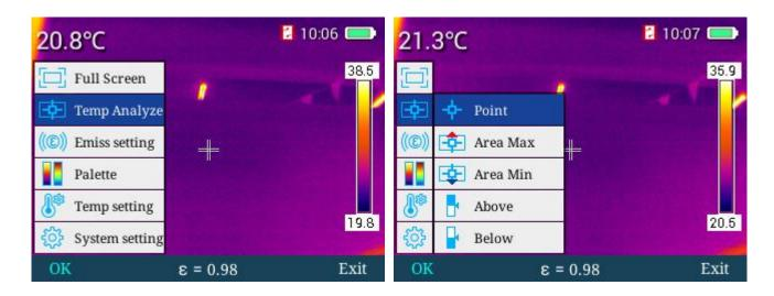
Test temperature of central point in "point" analysis mode, as shown below
