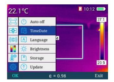
In "time and date" menu, press "▶" to successively select values to be adjusted which will be highlighted in blue, and then select "+" or "-" keys to adjust values selected. Press "◀" key to back to previous value selected and press "confirm" key to save current value adjusted, as shown below.
