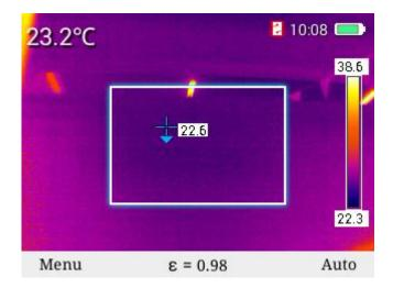
In "upper isotherm" mode, select high-temperature color band with "+" and "-" keys and display it in red. Meanwhile, display corresponding high temperature area in real-time image, as shown below.
