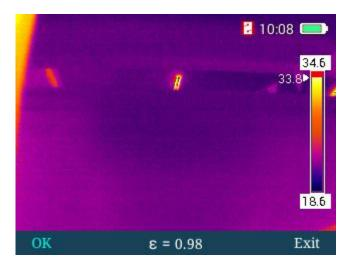
In "lower isotherm" mode, select low-temperature color band with "+" and "-" keys and display it in blue. Meanwhile, display corresponding low temperature area in real-time image, as shown below.
