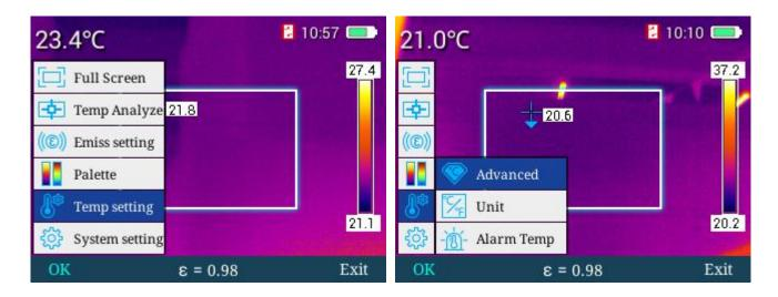
Then press "confirm" key or ">" key to go to "advanced" menu where you can adjust numerical values of reflected temperature, relative humidity and temperature measurement distance, as shown below.
