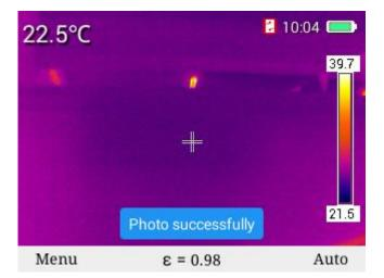
In fusion mode, you can adjust fusion position of infrared light and visible light. Press "confirm" key to go into fusion image adjustment mode, press four direction keys to displace visible light images and fuse visible light images with IR images, and press "confirm" key to store displacement adjustment setting.
