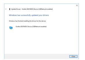
9、after the driver installation is complete, enter in the Device manager, in the network adapter ,you can find"Kindle USB RNDIS Device" ,means driver installation is complete;
