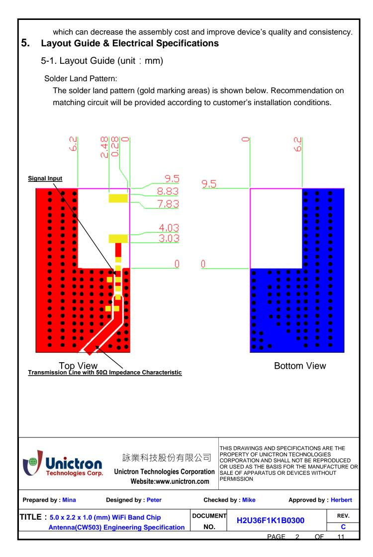
5-2. Electrical Specifications (Evaluation Board Dimensions: 40 x 40 mm<sup>2</sup>) 5-2-1. Electrical Table (2400~2500 MHz Band)
