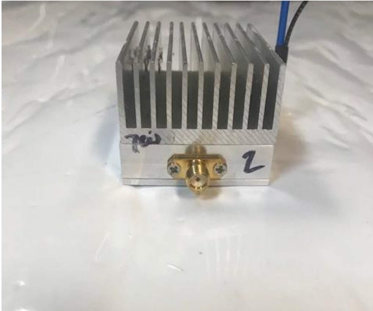
Figure 4. SAFE-1001 (700/800 MHz Amp) Side 2
