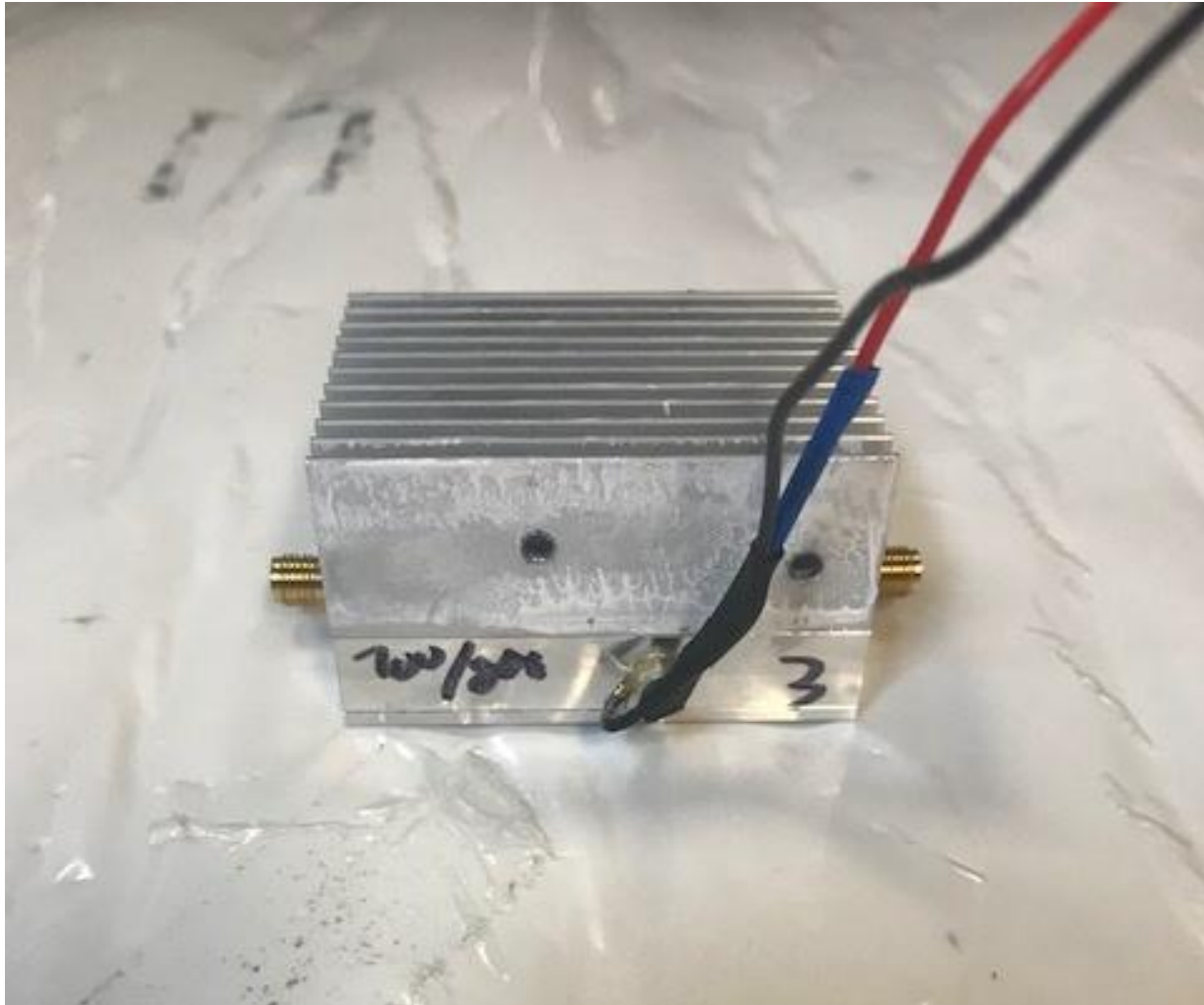
Figure 5. SAFE-1001 (700/800MHz Amp) Side 3
