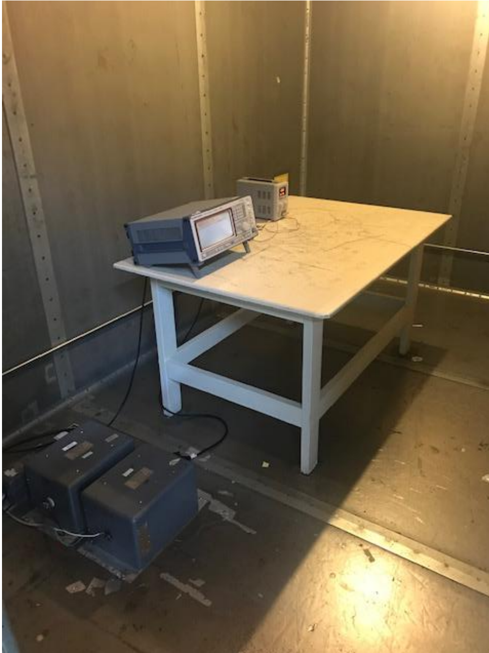
Figure 11. UHF EUT, Conducted Emissions, Set-Up Photo 1
