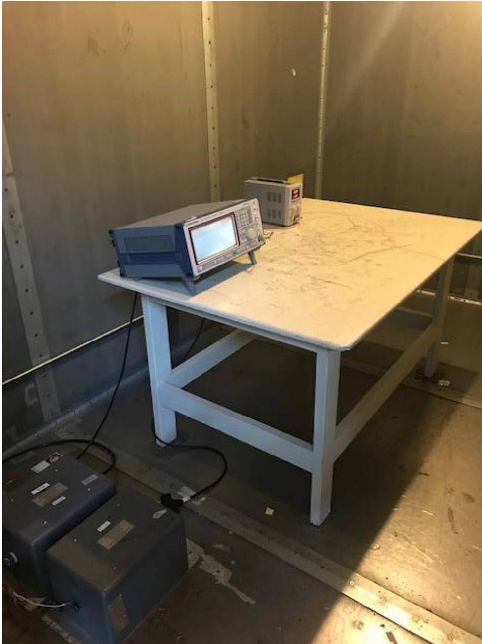
Figure 5. 700 – 800 MHz EUT, Conducted Emissions, Set-Up Photo 1
