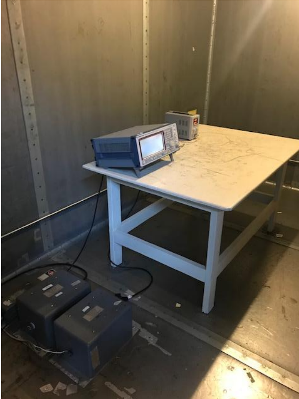
Figure 17. VHF EUT, Conducted Emissions, Set-Up Photo 1
