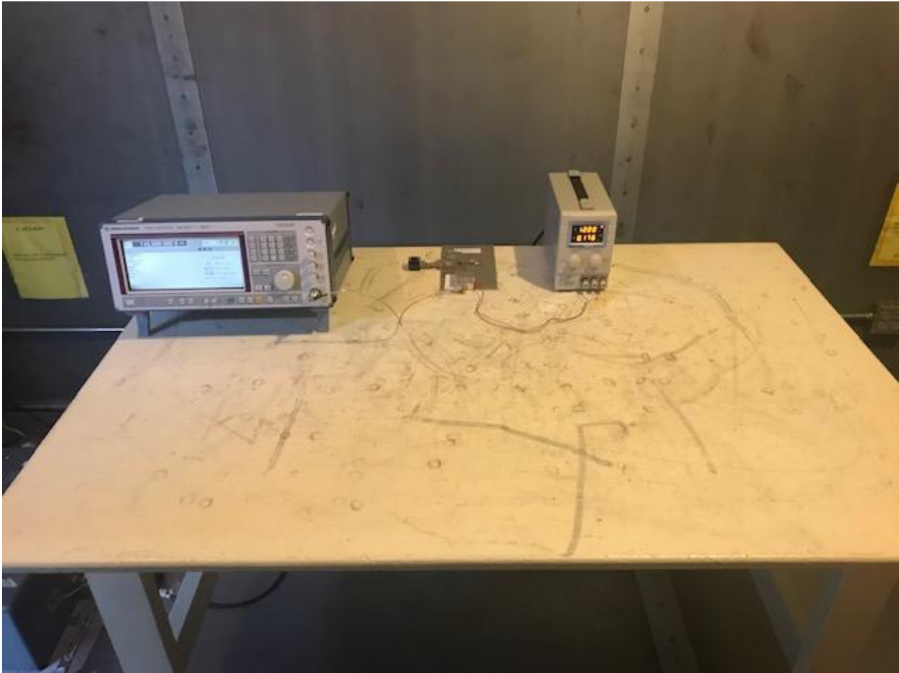
Figure 18. VHF EUT, Conducted Emissions, Set-Up Photo 2
