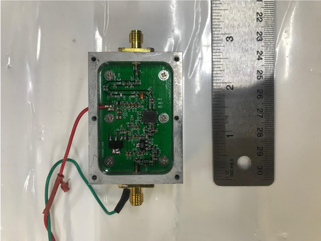
Figure 3. UHF Unit, Shield Removed
