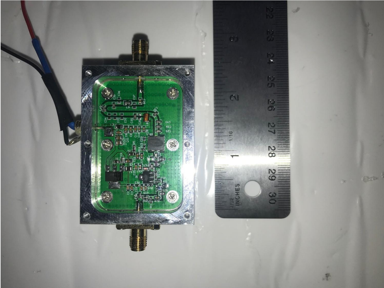
Figure 1. 700-800 MHz Unit, Shield Removed
