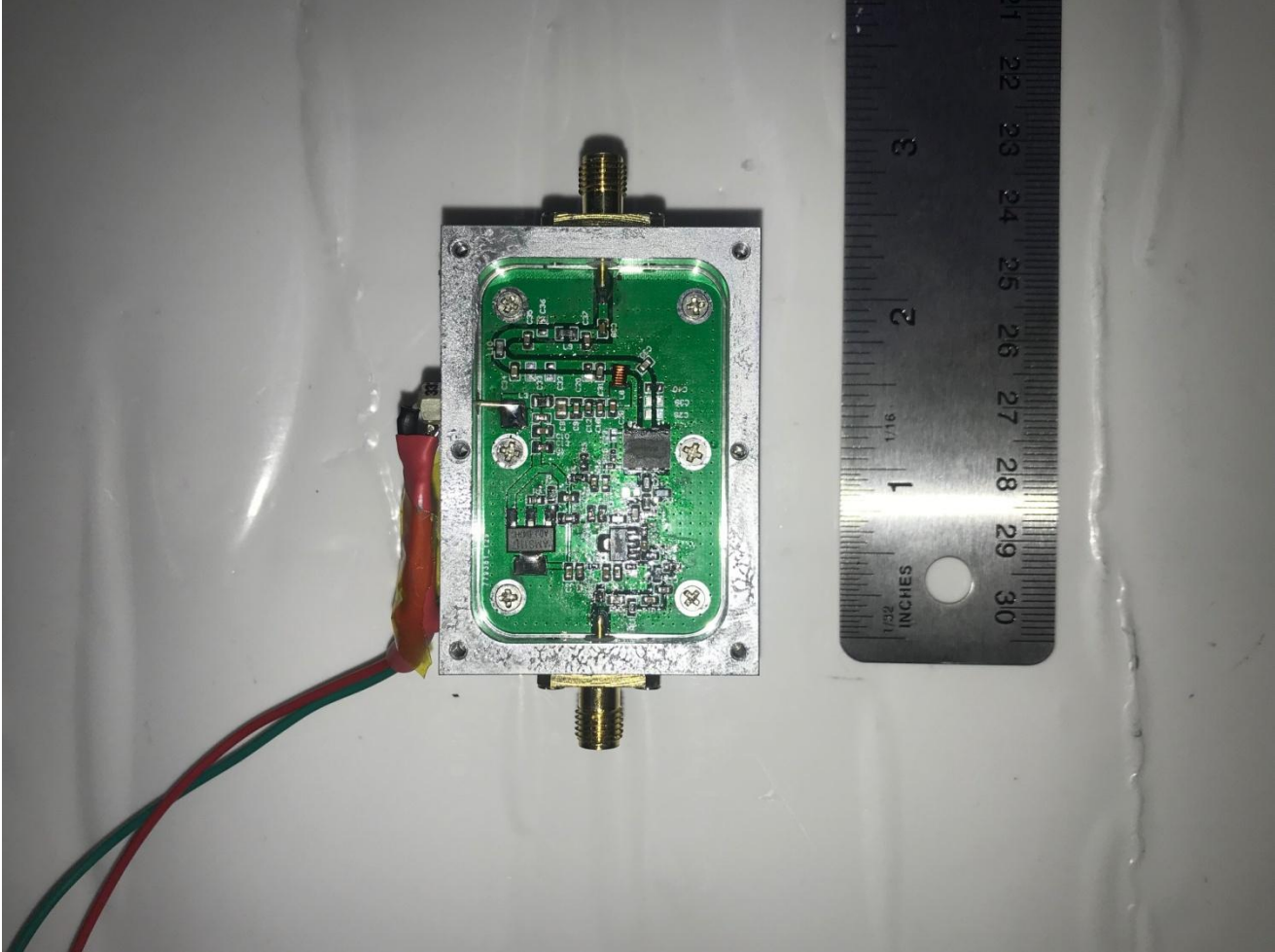
Figure 4. VHF Unit, Shield Removed
