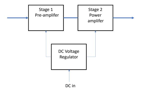
Note: There are no internal oscillators or clock frequencies in the SAFE-1001 amplifier
