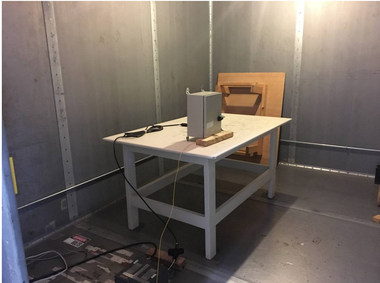
Figure7. Power Line Conducted Emissions Test Setup
