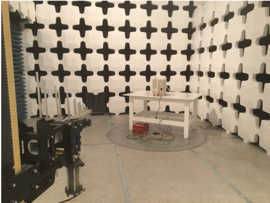
Figure 3. Radiated Emissions Test Setup, 200 MHz to 1GHz
