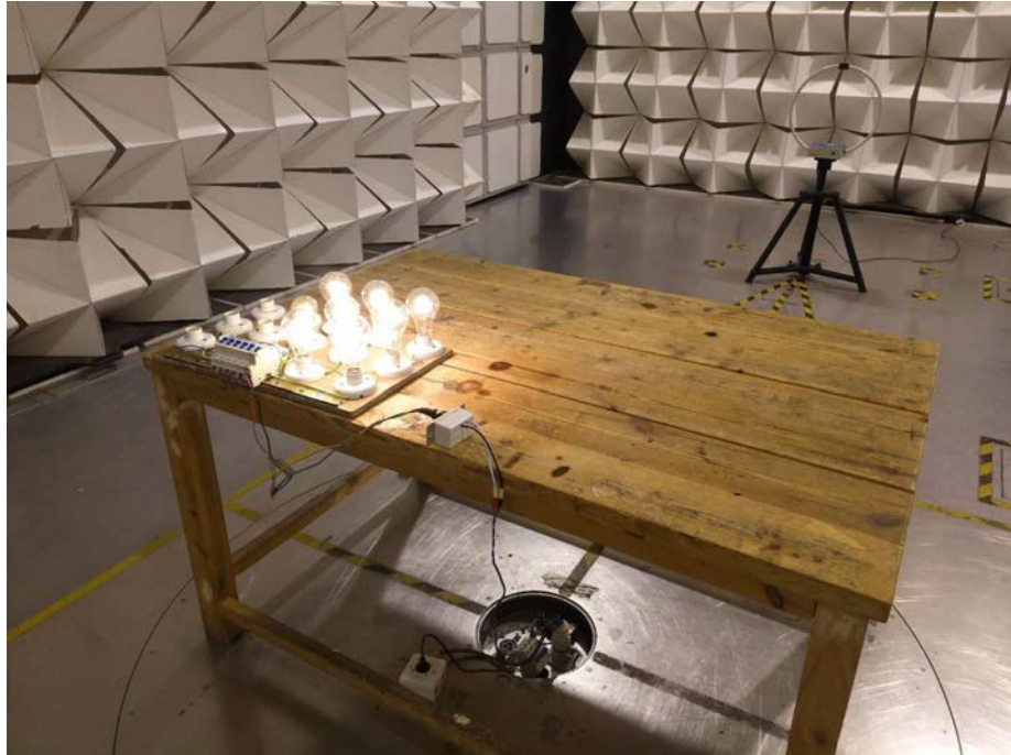
Test frequency from 30MHz to 1GHz
