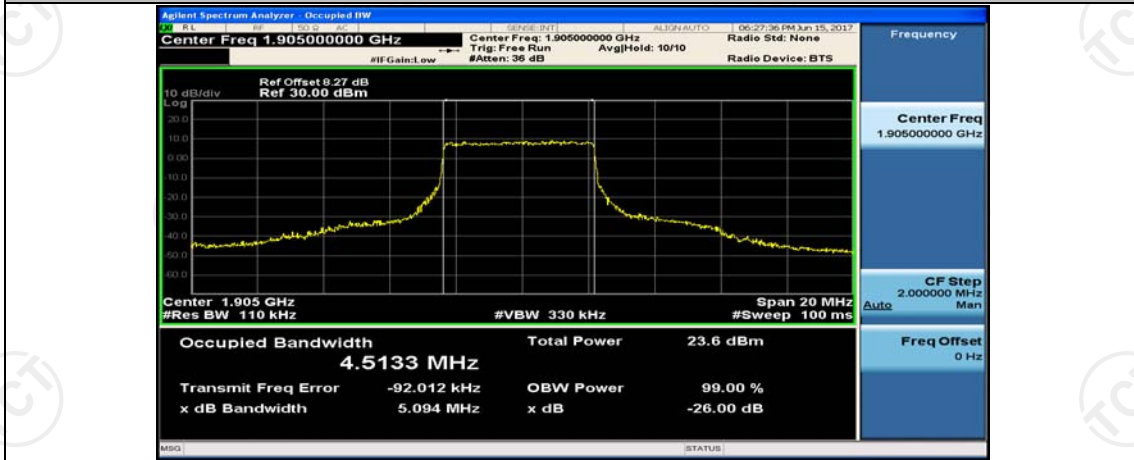
Channel Bandwidth: 10 MHz_HCH_QPSK_25RB#25
