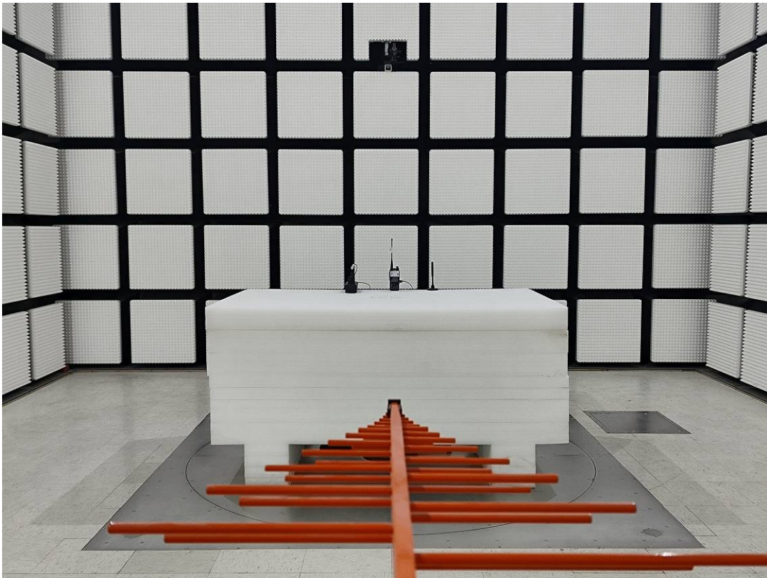
Radiated Emission Below 1GHz Rear View M2
