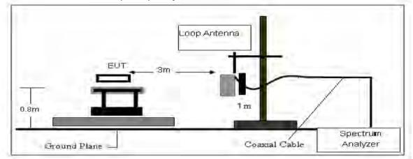
(B) Radiated Emission Test-Up Frequency 30MHz~1GHz
