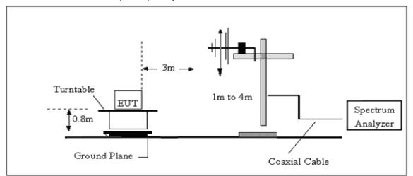
(C) Radiated Emission Test-Up Frequency Above 1GHz
