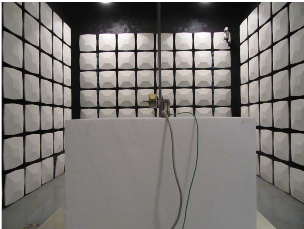
Radiated Disturbance Test Setup View-Above 1GHz
