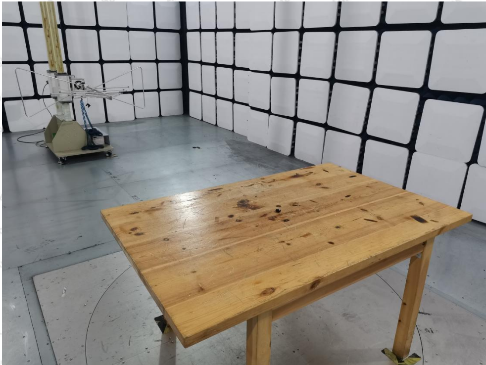
Photo of Radiation Emission Test
