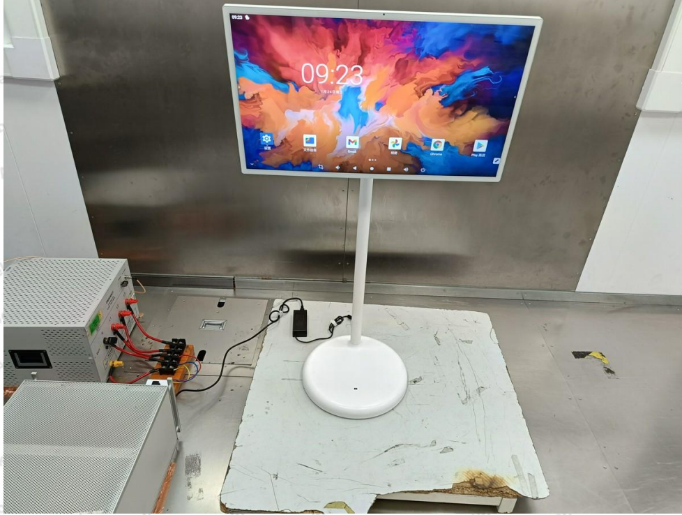
Photo of Radiation Emission Test (below 1GHz)
