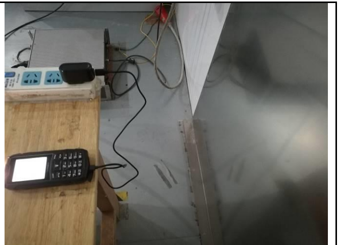
Conducted Emissions Test Setup – Side View
