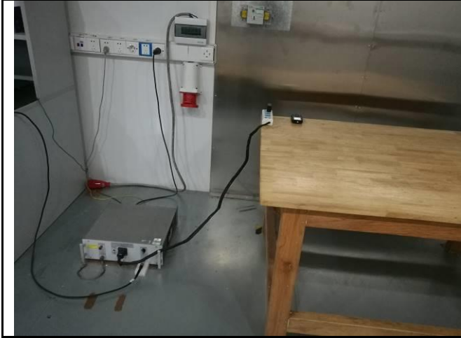
Conducted Emissions Test Setup Front View
