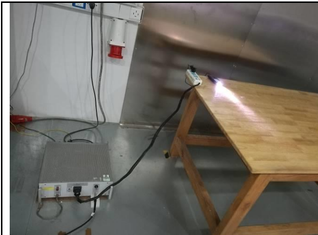
Conducted Emissions Test Setup – Front View
