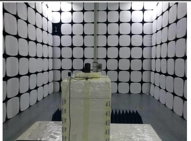
Radiated Spurious Emissions Test Setup Above 1GHz
