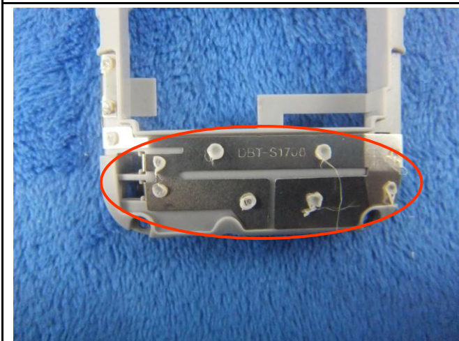
GSM/PCS Antenna View
