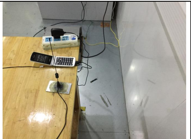
Conducted Emissions Test Setup Side View
