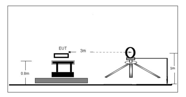
(B) Radiated Emission Test-Up Frequency 30MHz~1GHz
