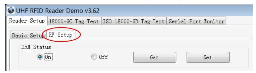
Note: If DRM was opened, the sensitivity of the reader will reduce significantly. So users could start this function according to the actual situation.
